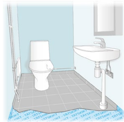
B4.6.2a Pipe penetrations in toilet room floors.
