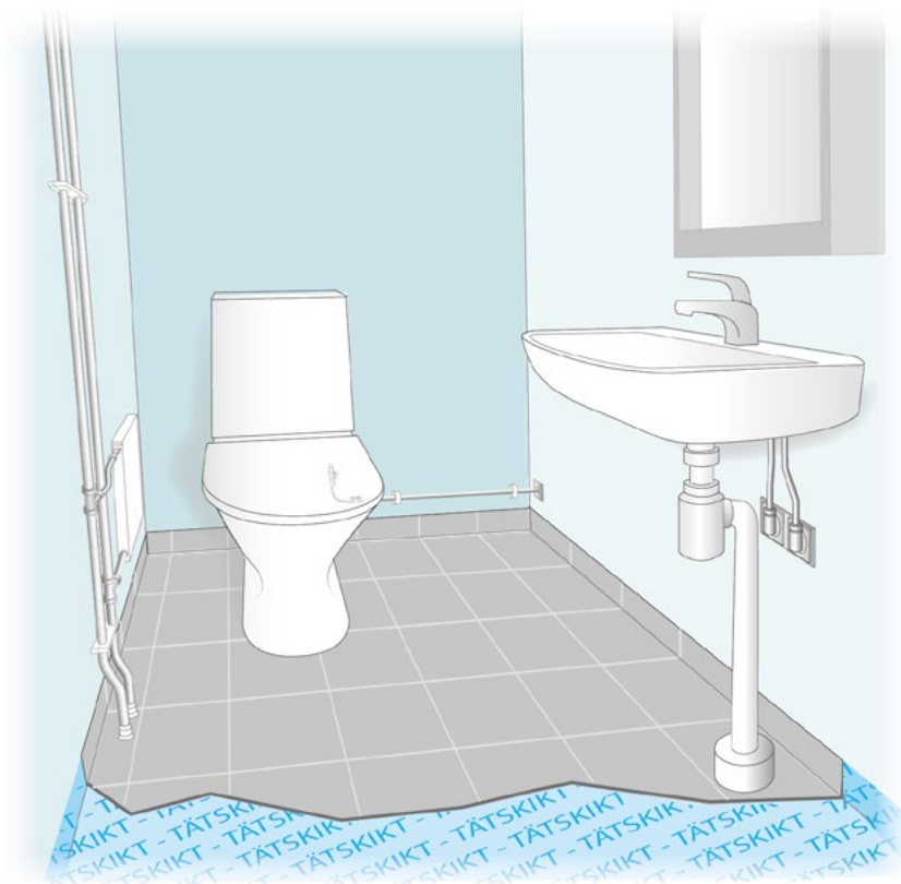
4.6.2a Pipe penetration in toilet room floor.
