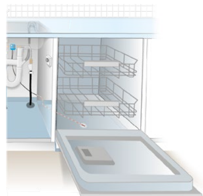
4.3.1a Example of a dishwasher with a leakage breaker and easily accessible operating element.
